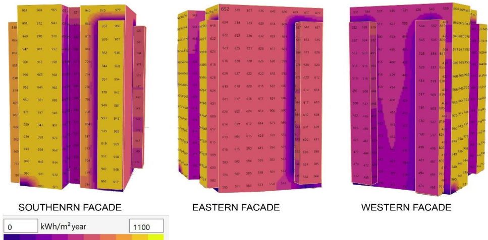
Figure 15. Detailed solar radiation mapping of Building A (Southern, Eastern and Western facades)
